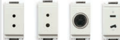
16300.B 2P 6 A 24 V (SELV) for 01620 plug. Depth: 26 mm 16301.B 2P 6 A 24 V (SELV) for 01616 / 01617 plugs. Depth: 26 mm 16332.B 5-pole DIN 41524. Depth: 10,5 mm 16345.B 2P 6 A 24 V (SELV), polarized. Depth: 26 mm
