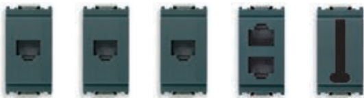
16335 RJ11, 6-position/4-conductor (6/4). Depth: 33,5 mm 16336 RJ12, 6-position/6-conductor (6/6). Depth: 33,5 mm 16337 RJ45, 8-position/8-conductor (8/8). Depth: 33,5 mm 16338 Double RJ11, 6-position/4-conductor (6/4). Depth: 31 mm 16347 8-contact, French standard. Depth: 21,5 mm
