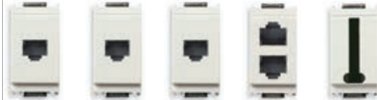
16335.B RJ11, 6-position/4-conductor (6/4). Depth: 33,5 mm 16336.B RJ12, 6-position/6-conductor (6/6). Depth: 33,5 mm 16337.B RJ45, 8-position/8-conductor (8/8). Depth: 33,5 mm 16338.B Double RJ11, 6-position/4-conductor (6/4). Depth: 31 mm 16347.B 8-contact, French standard. Depth: 21,5 mm
