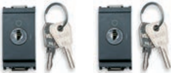
16165 2P 16 AX 1-way switch 16165.S As above, key removable in 'O' (OFF). Depth: 32,5 mm 16185 2P NO 16 A push button. Depth: 32,5 mm
